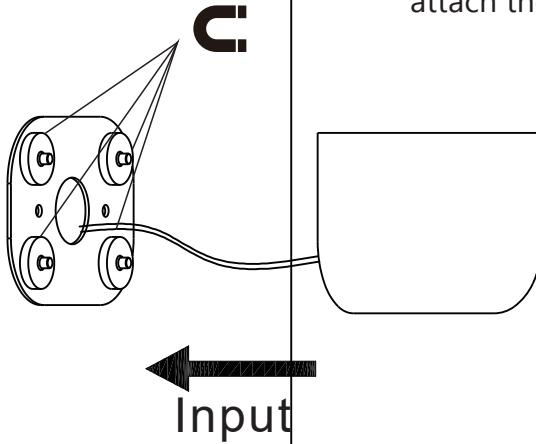
Align with the magnetic position and attach the lamp body by adsorption.
