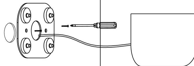
Tighten the backplate with mounting screws and connect the wires
